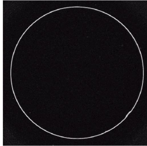
An image of a contact lens which is enhanced in order to make defects (at four and five o'clock in the image) more obvious
